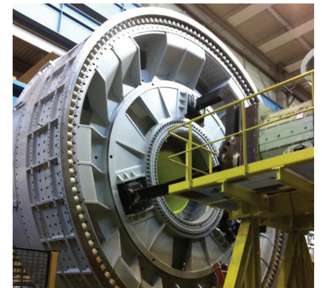
■ Figure 4 | A GE Haliade 6 MW generator on test | Courtesy of GE Vernova/Stuart Bradley
