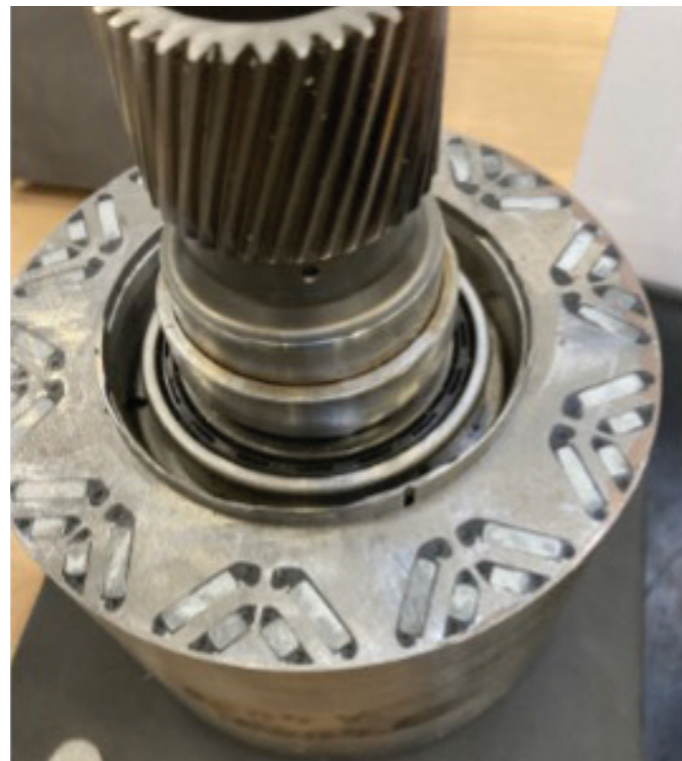
■ Figure 17 | An automotive IPM rotor showing the magnets and their encapsulation | Photo from WMG, University of Warwick
