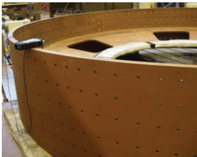
Figure 8 | A direct-drive generator rotor wheel showing the magnet carrier threaded holes to suit two magnet carrier assemblies | Courtesy of GE Vernova/Stuart Bradley
