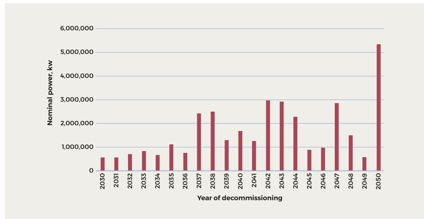
Figure 13 | Graph showing the decommissioning of turbines (onshore and offshore) by nominal power rating and year. The nominal power rating is the electrical output for continuous operation. The amount of magnet material is proportional to the nominal power rating, with a higher nominal power rating requiring more magnet material as a linear relationship – for example, a direct drive generator has between 800 and 1200 kg of magnet per MW of nominal power
